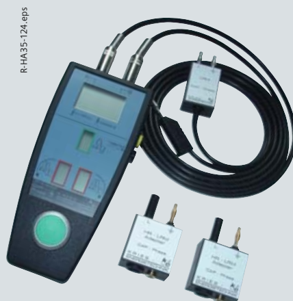
Phase comparison test unit make Kries, type CAP-Phase as combined test unit (HR and LRM) for: – Voltage detection – Repeat test – Phase comparison – Phase sequence test – Self-test The unit does not require a battery
