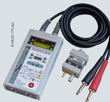
Phase comparison test unit make Hachmann, type VisualPhase LCD as combined test unit (HR and LRM) for: – Voltage detection with measured-value indication – Interface test – Low voltage detection – Documentable repeat test – Phase comparison with LED signal and measured-value indication – Phase angle from -180^\circ to +180^\circ – Phase sequence evaluation – Frequency quality – Complete self-test
